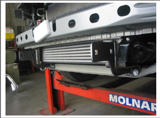
Figure 9: ECB steel mounting brackets fitted.
