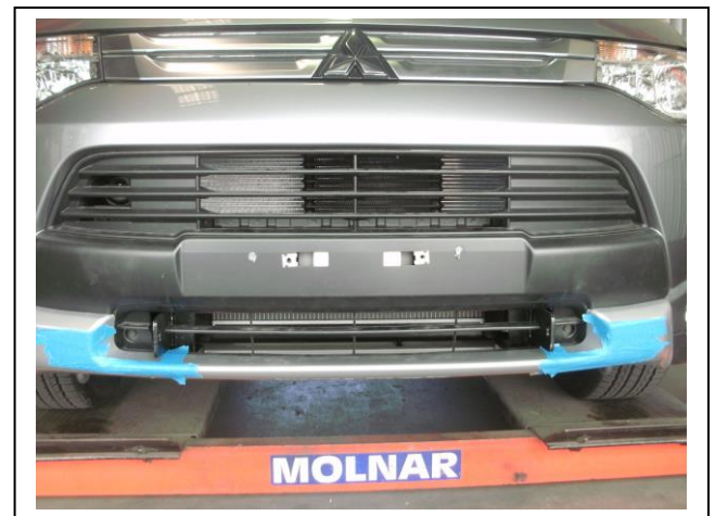
Figure 12: ECB steel mounting brackets with bumper fitted.
