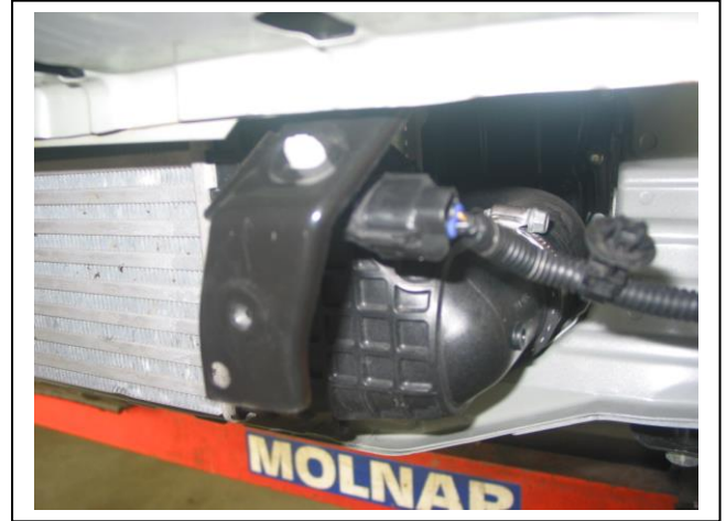
Figure 10: Temperature sensor on bumper locator.
