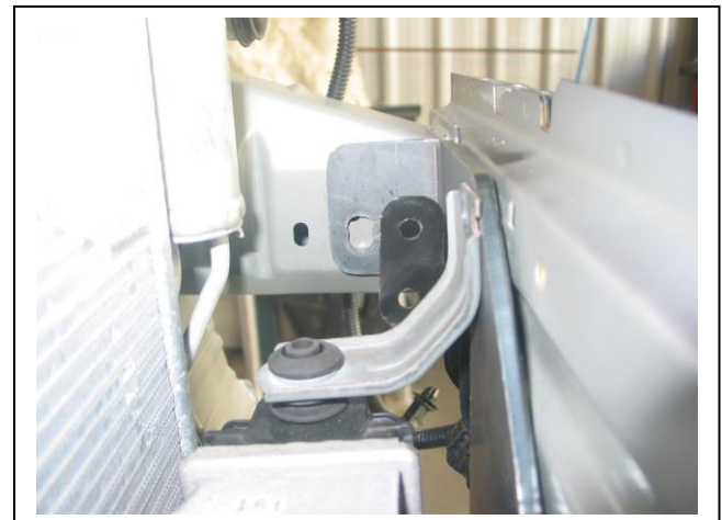
Figure 8: Flattened tab on top intercooler mount
