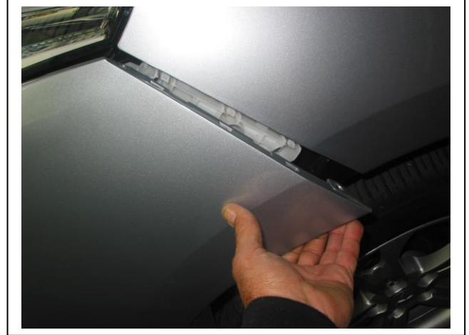
Figure 4: Carefully remove bumper from guard clips
